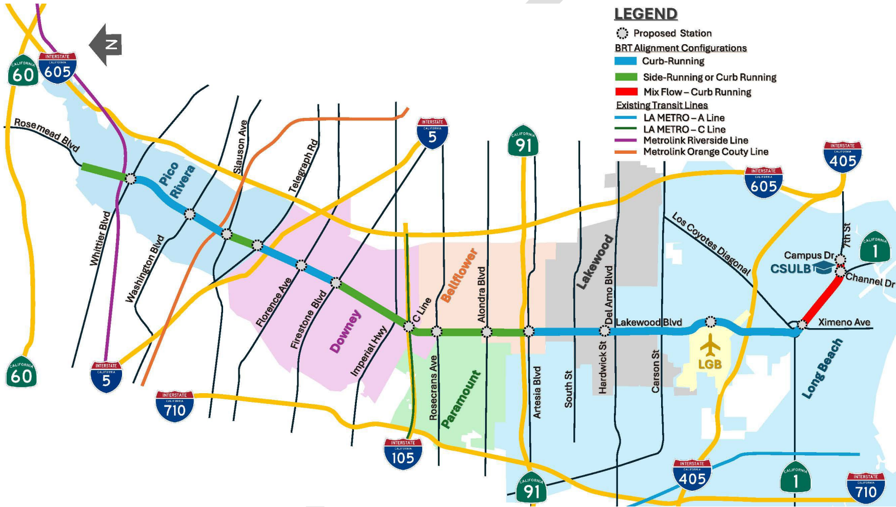
Figure 5-11. BRT Alignment Configuration
